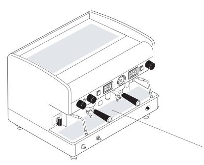
The nameplate of the machine is fixed on the base of the frame under the drain pan.
